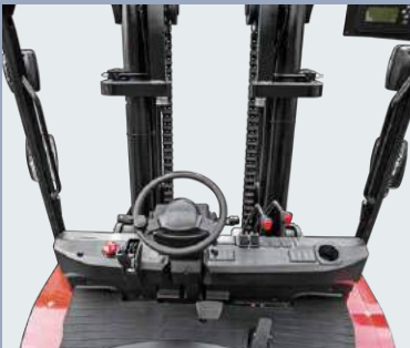
New designed broad view mast provides better forward view ability
