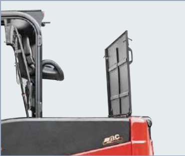
Full opened battery cover is easy for battery service
